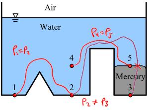
2. The pressure at any free surface open to the atmosphere is atmospheric pressure,  $P_{\text{atm.}}$
