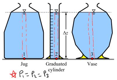
Consider the three containers in the figure. At first glance, it may seem that the pressure at point 1 is greater than that at point 2 since the jug of water weighs much more than the graduated cylinder of water. Others might argue that the pressure at point 3 is greater than that at point 2, since the weight of the water is more "concentrated" on the small area at the bottom of the vase. However, **all three pressures are identical**. Use of
