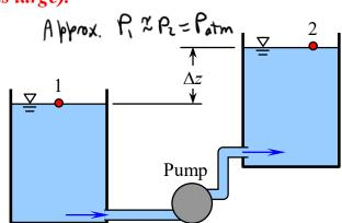
common to ignore the difference between  $P_1$  and  $P_2$ , and approximate both pressures as the same value of atmospheric pressure,  $P_{\text{atm}}$ .
