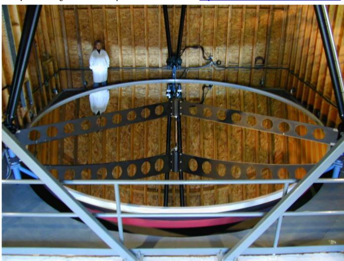
2. Mirrors made from spinning molten glass in a furnace, and letting it harden in the paraboloid shape.
