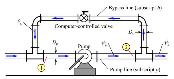
**To Do:** Calculate and plot how volume flow rates  $\dot{\mathcal{V}}_p$ ,  $\dot{\mathcal{V}}_b$ , and  $\dot{\mathcal{V}}_d$  vary with the minor loss coefficient of the value as it goes from fully open ( $K_{L, \text{ value}} = 0.2$ ) to fully closed ( $K_{L, \text{ value}} \rightarrow \infty$ ).
