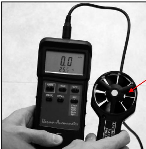
Turbine used for measurement of air speed
