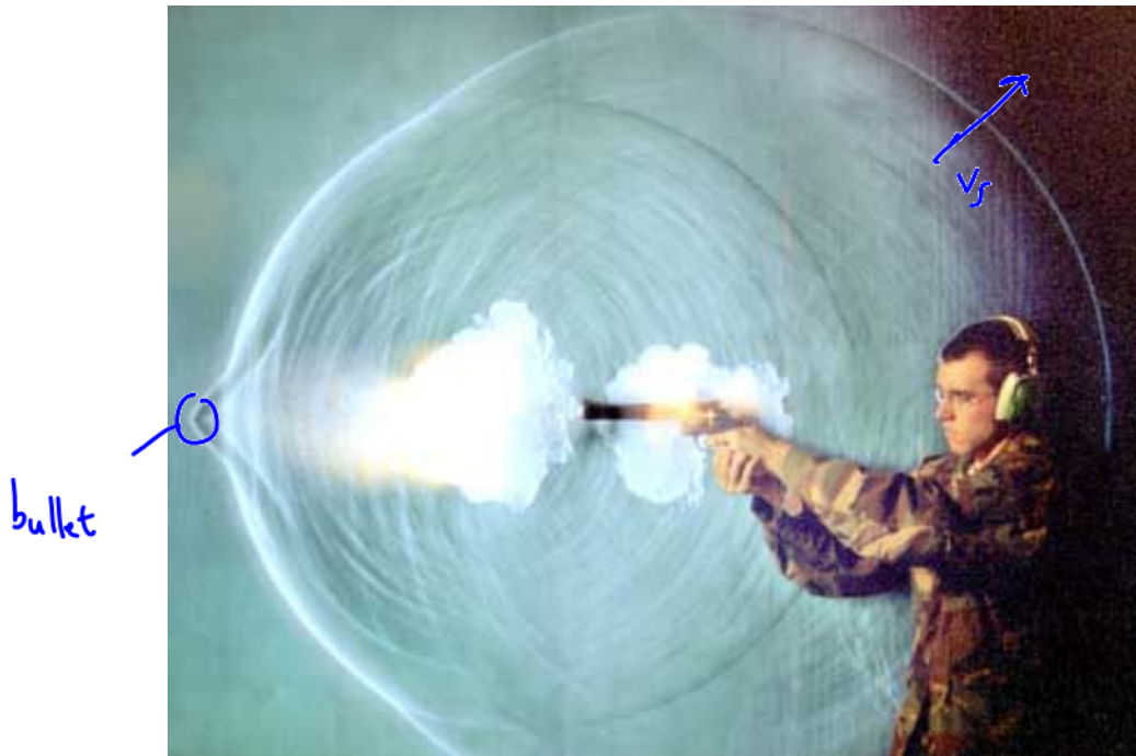
Spherical shock from an explosive gun shot; bullet emerging on left.
