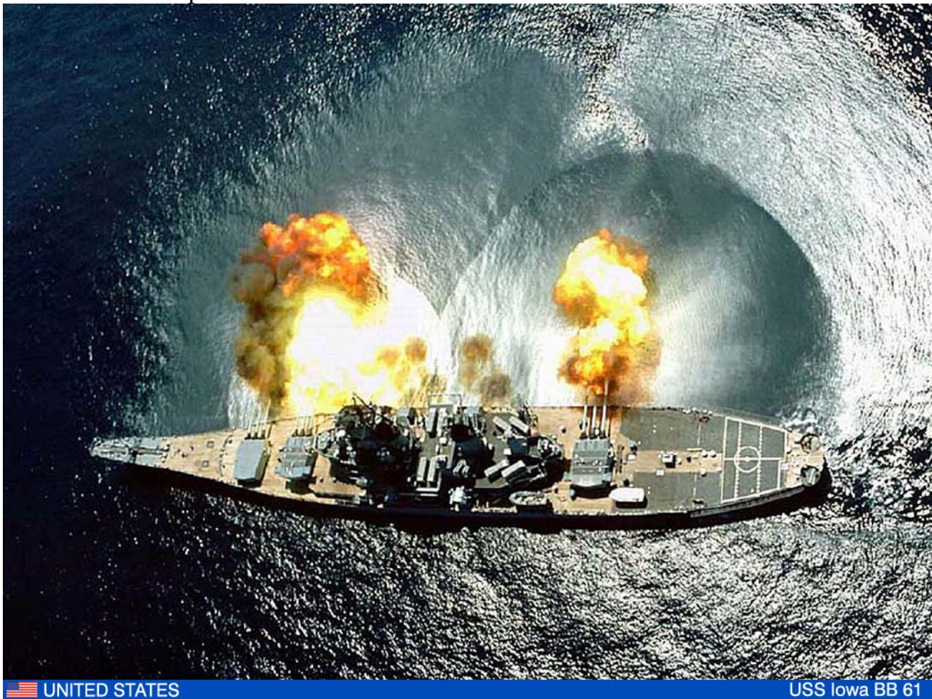
Guns shooting from the USS Iowa; shocks seen on water surface!
