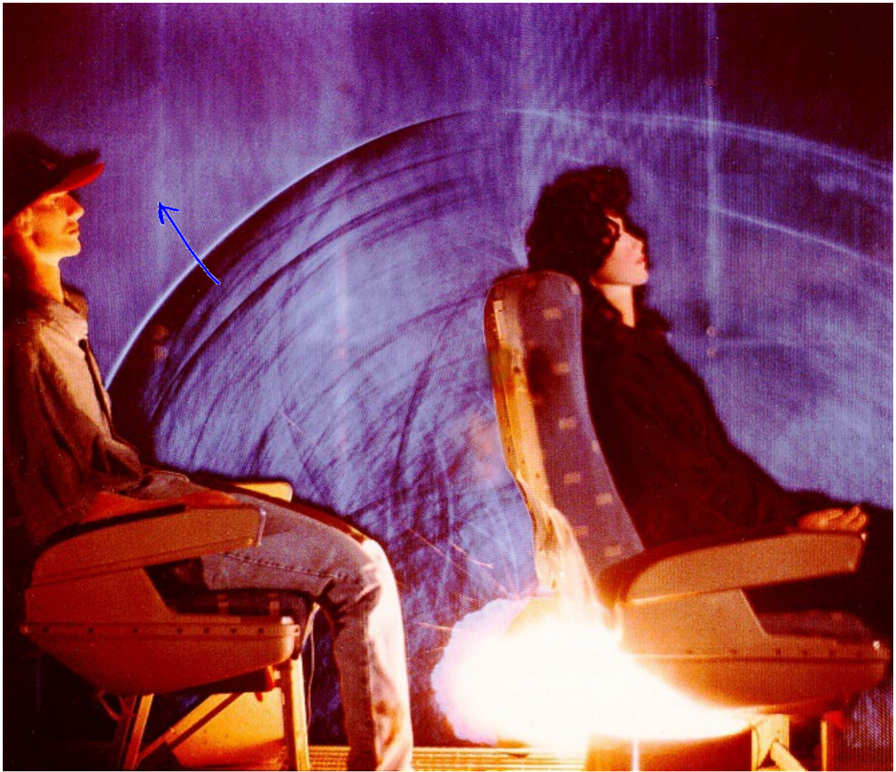
Color schlieren image of an explosion beneath a full size aircraft seat occupied by a dummy. This photo aided in the research (funded by the FAA) of aircraft hardening in response to incidents of international terrorism. Photos courtesy of G. S. Settles.
