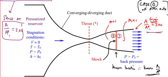
To do: Calculate the pressure and Mach number at the exit plane.
