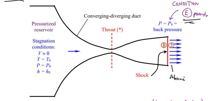
To do: Calculate the pressure and Mach number at the exit plane. (downstrain of thek) Solution:
