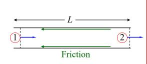
**<u>To do</u>**: Estimate the maximum possible duct length that will not affect the inlet conditions.
