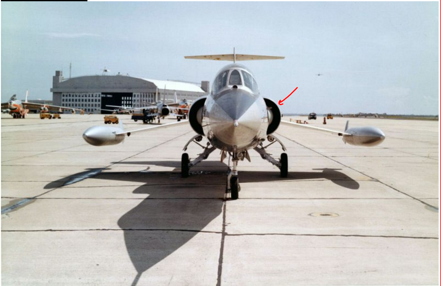
F-104 Starfighter: Half-round inlets with halfcones.
