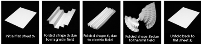
Figure 1: A CONCEPT FOR A MULTI-FIELD RESPONSIVE ORIGAMI STRUCTURE THAT ACTIVELY FOLDS FROM AN INITIALLY FLAT SHEET TO COMPLEX THREE-DIMENSIONAL SHAPES IN RESPONSE TO DIFFERENT APPLIED FIELDS. IT IS ALSO CAPABLE OF ACTIVELY UNFOLDING FROM ANY SHAPE BACK TO THE FLAT SHEET.
